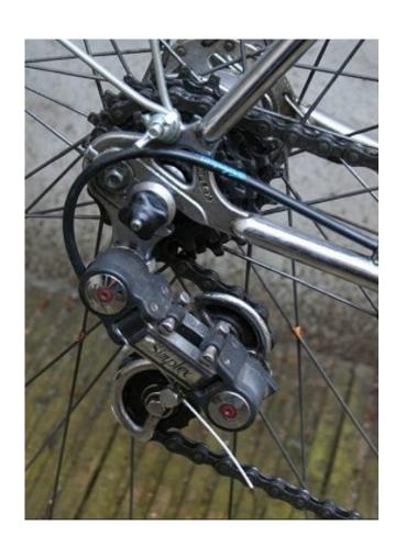
The original plastic rear derailleur was a bit flexible and a bit fragile, so a new version was introduced with metal reinforcing plates in the arms and more robust spring housings
