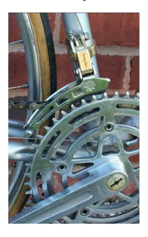
Aluminium alloy construction (steel cage)
